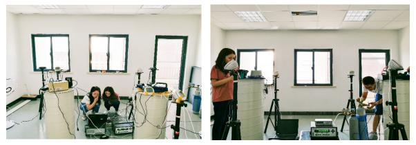
Figure 2.2. IAQ measurements in the P+ building comprising measurement of VOCs, PM2.5, thermal and humidity conditions as well as energy performance (Source: Student work, Nanjing University)
