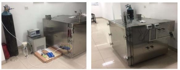
Figure 2.1.New small-scale environmental chamber systems at Nanjing University, China. (Source: Student work, Nanjing University)
