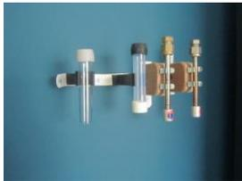
Passive sampling (VOCs, O<sub>3</sub>, NO<sub>2</sub>)
