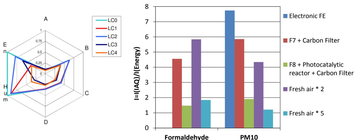
Figure 2. Accounting for energy consumption in IAQ evaluation (left graph: *A*, *B*, *C* and *D* are IAQ indices, *Hum* is relative to humidity and *En* is the energy index, 0 is the best situation for IAQ and energy; right graph: the index aggregates IAQ and energy, 0 is the worst situation because of bad IAQ, high energy consumption or both).
