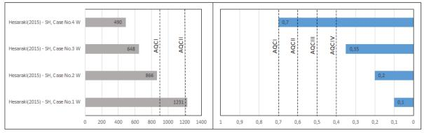
Figure 1. Average CO<sub>2</sub> concentrations (ppm) vs whole house-ventilations rates (ACH) compared to air quality classes defined by EN 15251 (Hesaraki, 2015)
