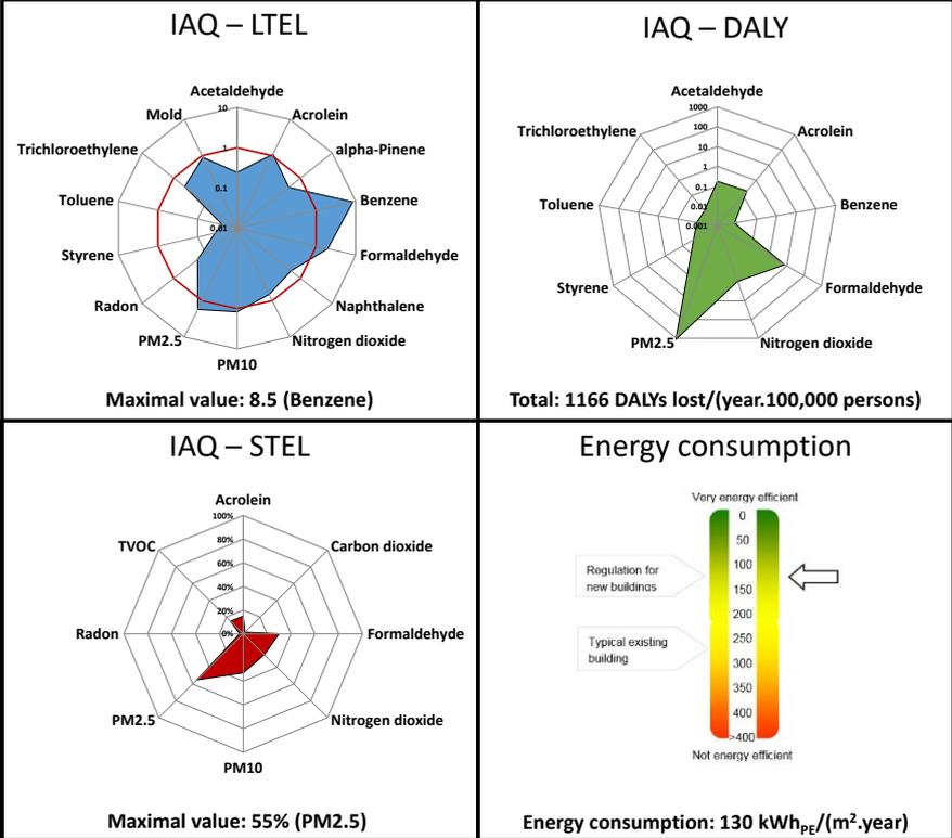
Figure 1: IAQ/Energy dashboard for low-energy residential buildings – IAQ-LTEL is for Indoor Air Quality – Long-Term Exposure Limit, IAQ-STEL is for Indoor Air Quality – Short-Term Exposure Limit and IAQ-DALY is for Indoor Air Quality – Disability-Adjusted Life Years (data represented here are just for display and do not represent actual situation).
