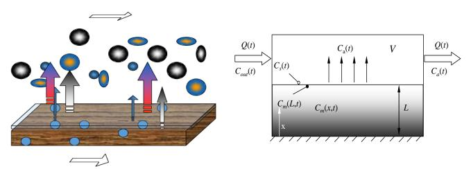
Figure 2. Schematic illustration of pollutant emission from dry materials.
