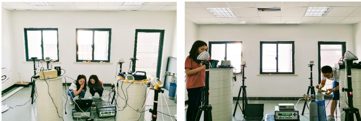
Figure 2.2. IAQ measurements in the P+ building comprising measurement of VOCs, PM2.5, thermal and humidity conditions as well as energy performance (Source: Student work, Nanjing University)
